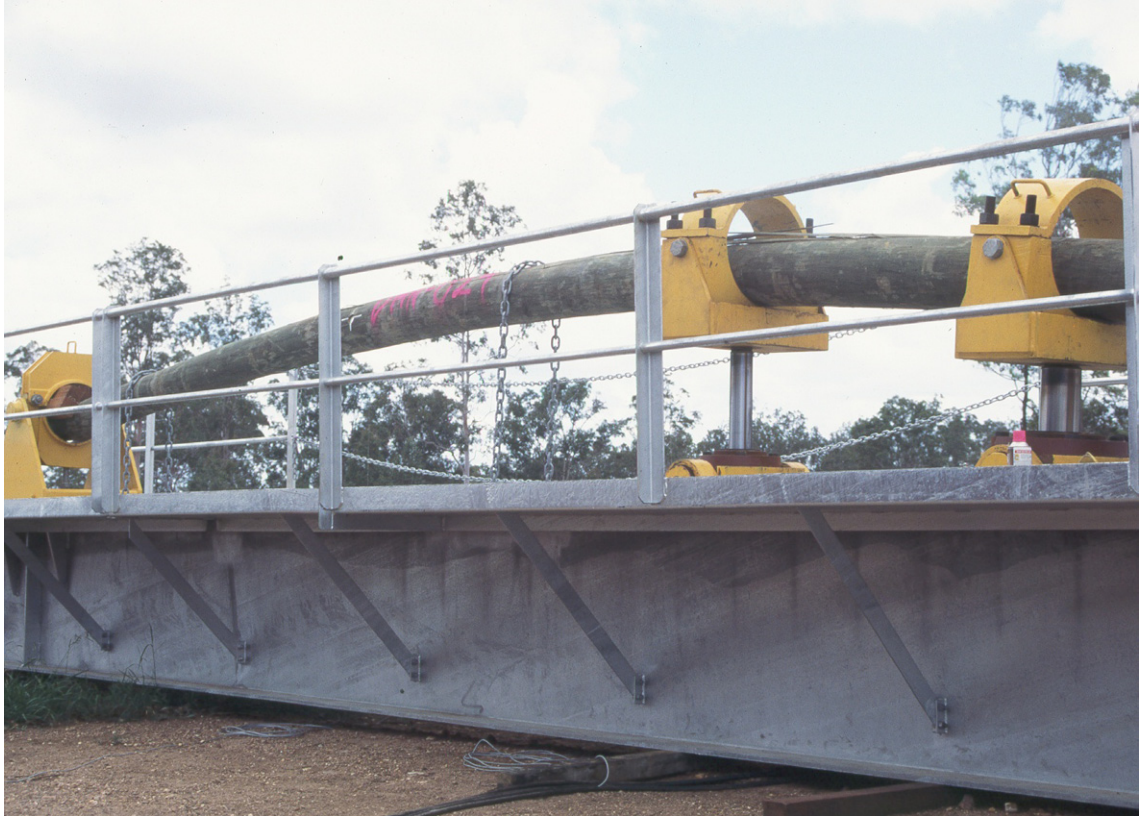
Figure D.2 — Example of four-point bending test procedure
