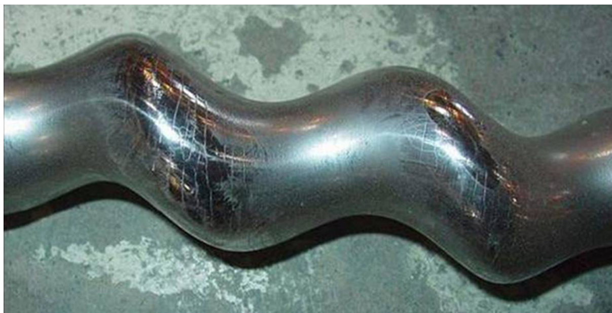
Figure I.3 — Cracked/heat cracked rotor (provided courtesy of Kudu Industries)
