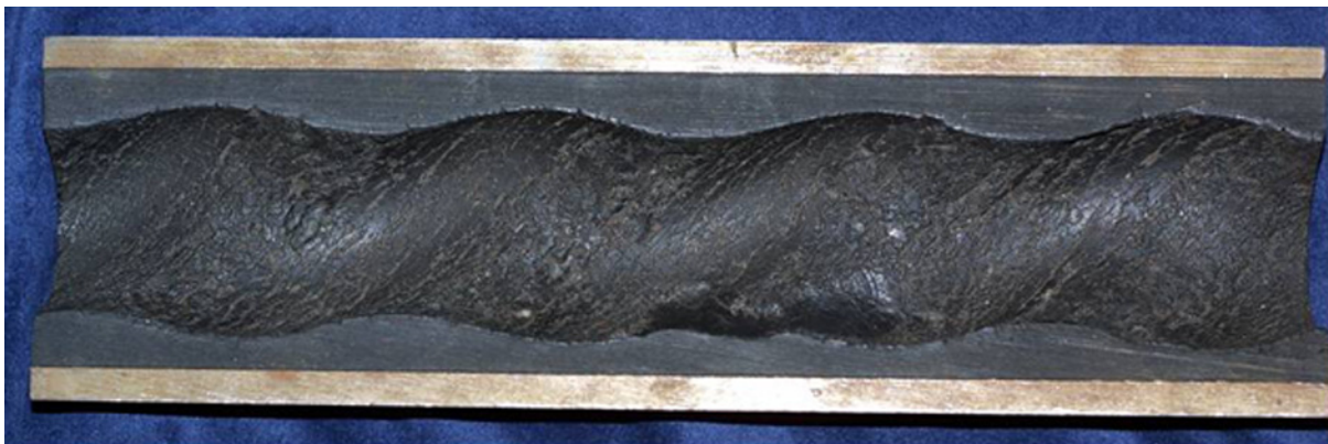
Figure I.6 — Burned/overheated stator (provided courtesy of CFER Technologies)
