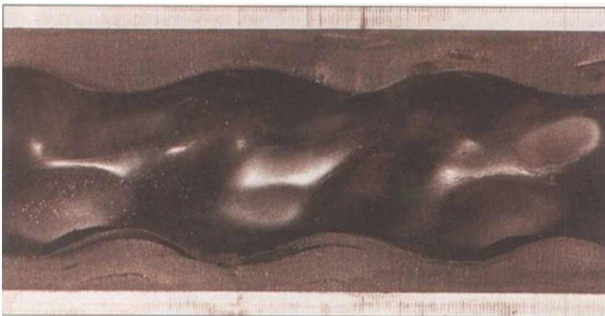
Figure I.5 — Blistered stator (provided courtesy of Weatherford)
