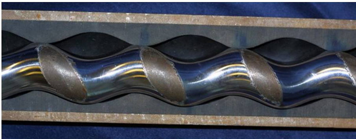
Figure I.2 —Worn rotor (provided courtesy of CFER Technologies)
