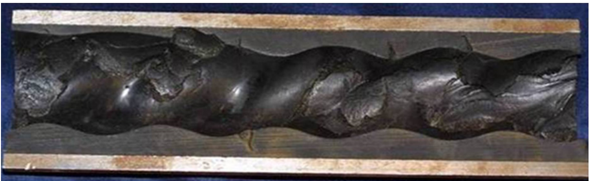
Figure I.10 — Torn/chunked stator (provided courtesy of CFER Technologies)
