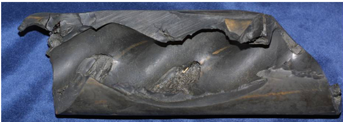
Figure I.8 — Debonded stator (provided courtesy of CFER Technologies)
