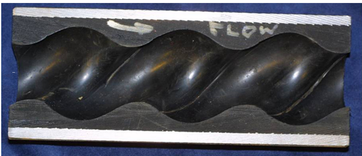
Figure I.7 — Eroded/pressure washed stator (provided courtesy of CFER Technologies)
