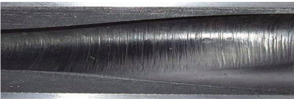
Figure I.12 — Stator worn (provided courtesy of Kudu Industries)
