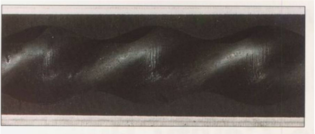
Figure I.9 — Scratched/grooved stator (provided courtesy of Weatherford)
