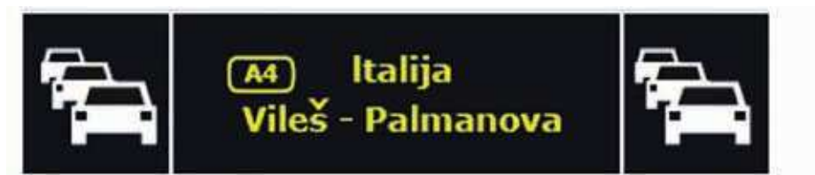
Figure D.5 — Example of a text VMS with one pictogram on each side
