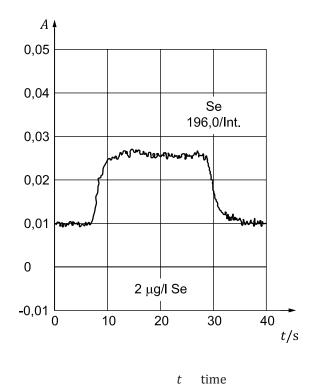
NOTE Background signal is made up of instrumental blank and reagent blank. When a sample is analysed, the signal from selenium in the sample is superimposed on the background level.
