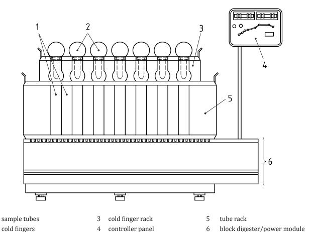
Figure B.3 — An example of a suitable block digester with the cold finger arrangement
