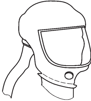
Figure A.10 — Examples of tight-fitting respiratory interfaces covering the head — Class dT
