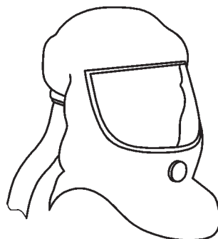
Figure A.9 — Examples of loose-fitting respiratory interfaces covering the head — Class dL
