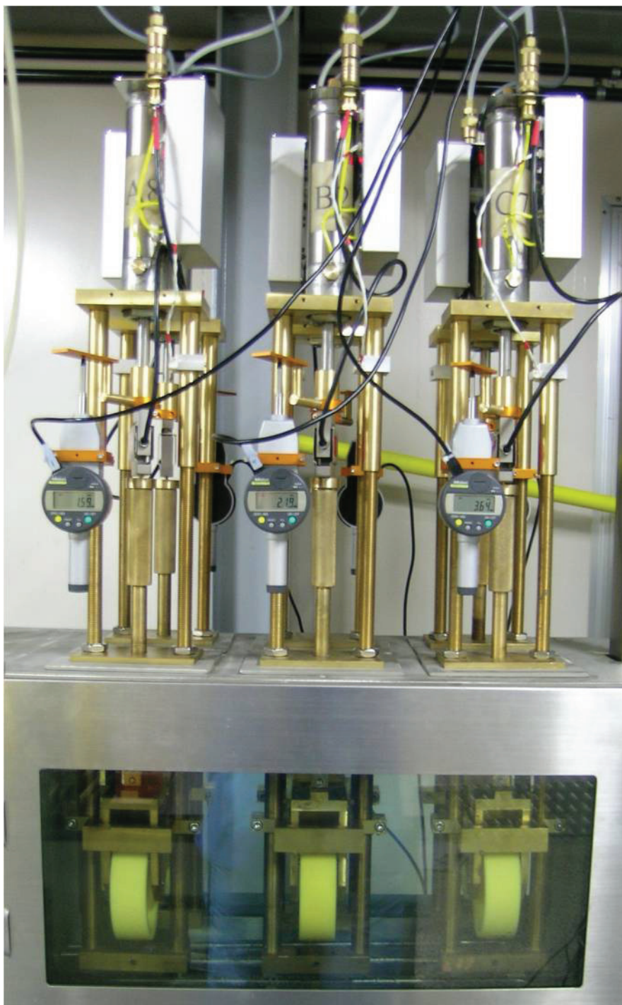
Figure A.5 — Pneumatically actuated notched ring loading device with electronic displacement gauge assembly
