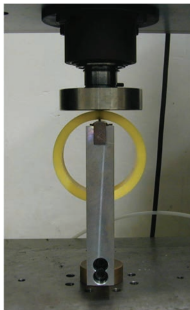
b) Notching on a universal testing machine
