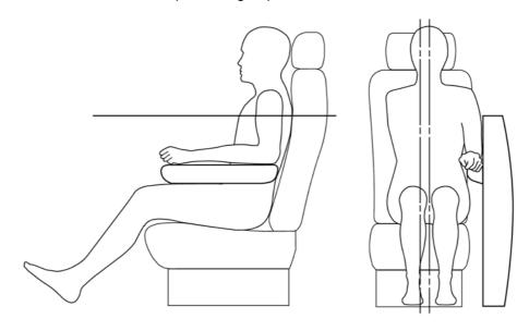
Figure 3 — Elbow on armrest — no gap between upper arm and door trim static deployment test (left-hand side shown)
