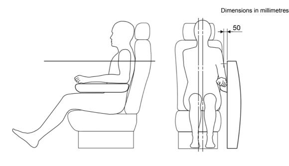
Figure 2 — Elbow on armrest — 50 mm gap between arm and door trim static deployment test (left-hand side shown)
