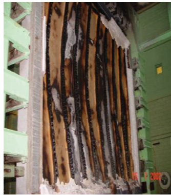
Figure A.1 —Behaviour and failure mode of wood-framed wall assembly
