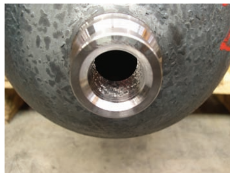
Figure A.14 — Chipped thread
