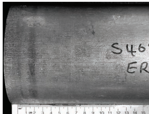
Figure A.7 — Blister (aluminium)
