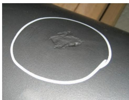
b) Metallic or scale impression
