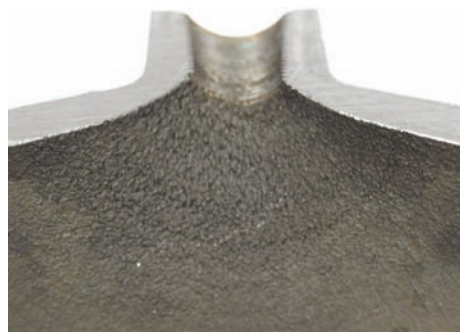
Figure A.13 — “Orange peel”
