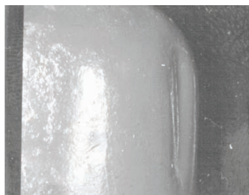
Figure A.4 — Dent containing cut or gouge
