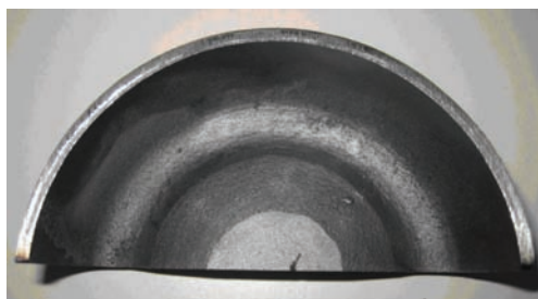
Figure A.10 — Cylinder shoulder folds or cracks before and after machining
