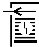
Figure A.9 — Example of a graphical representation denoting a feeder malfunction
