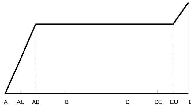
Figure 13 — Load sharing factor for cylindrical helical gears with \epsilon_{\beta} \geq 1 and optimum profile modification
