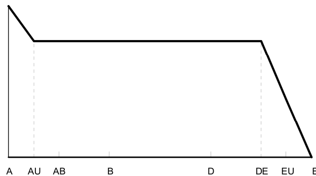
Figure 14 — Load sharing factor for cylindrical helical gears with \epsilon_{\beta} \geq 1 and optimum profile modification on the addendum of the driven gear and/or the dedendum of the driving gear
