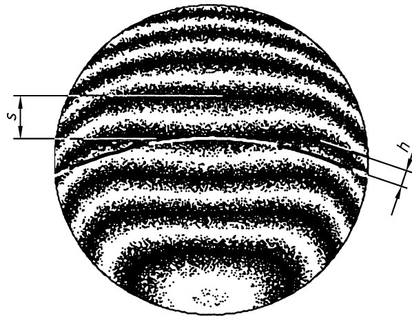
Figure A.5 — Example of an interferogram showing 0,3 wavelengths of rotationally invariant irregularity (evaluation in Example 5)
