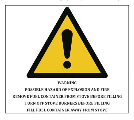
**8.5** Openings for filling fuel tanks shall be identified to indicate the type of fuel to be used with the system. The word "FUEL" alone shall not be used.
