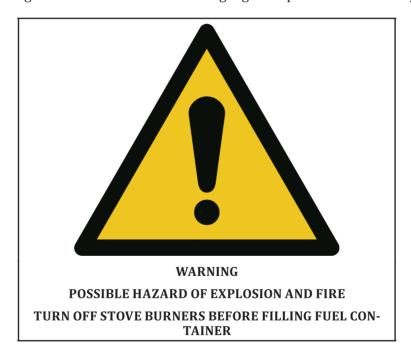
**8.4** Non-pressurized stoves with integral tanks, having fuel held in absorbent material, which are designed to have the fuel container removed for filling, shall have a permanent, legible warning label with the following informational elements in language acceptable in the country of use.
