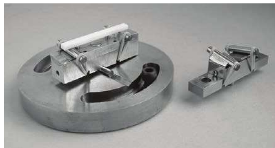
b) Schematic of a fixture with special cradles to hold the bearing rollers
