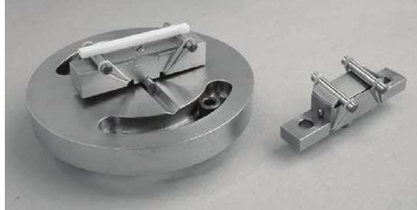
a) Inner pair of bearing rollers (on the right) are parallel and articulate together as a pair in a cradle assembly
