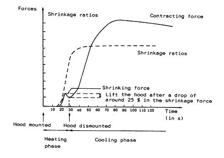
Figure 2 - Measurement of the forces and of the shrinkage ratio - Example of typical kinetics of the phenomena
