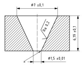
The value of surface roughness, Ra, is the mean height of the profile below and above the line, as defined in NOTE ISO 4287.
