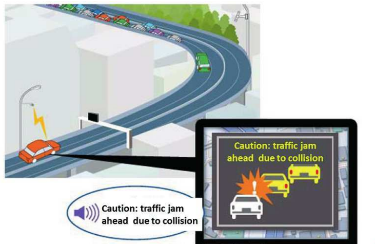
Figure D.7 — Traffic congestion warning
