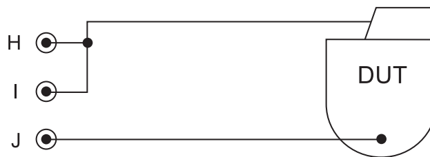
Figure 14 — Connection to a single-channel unipolar device
