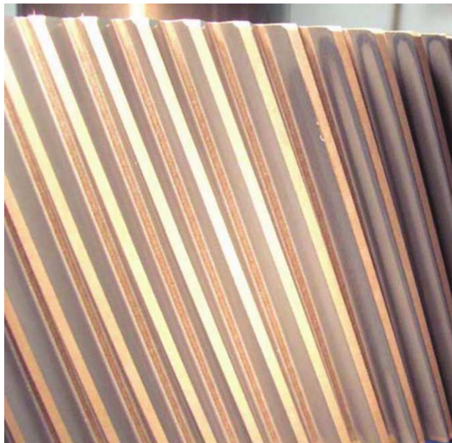
Figure 6 — Progressively worse surface temper of teeth from left with Class FA no tempering to right with Class FE rehardening surrounded by Class FD heavy tempering on four teeth at right
