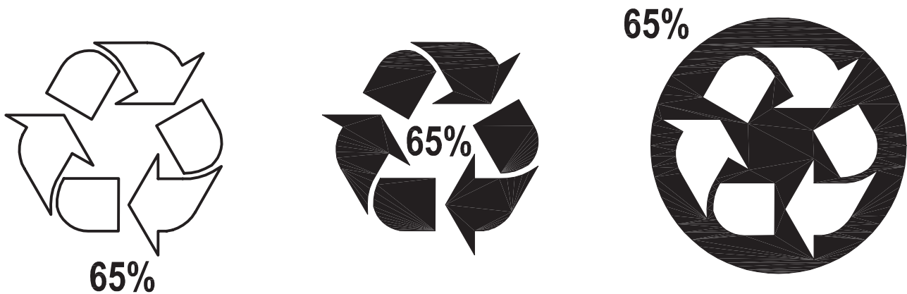
Figure 2 — Examples of acceptable locations of percentage value when using the Mobius loop to make claims about recycled content
