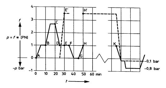
NOTE: The solid line represents the time limits for pressure changes (inclusive of constant values) and the dotted line represents the bending force, *F*, (exclusive of values). The lines do not infer that the rates of change of pressure or force are strictly linear.
