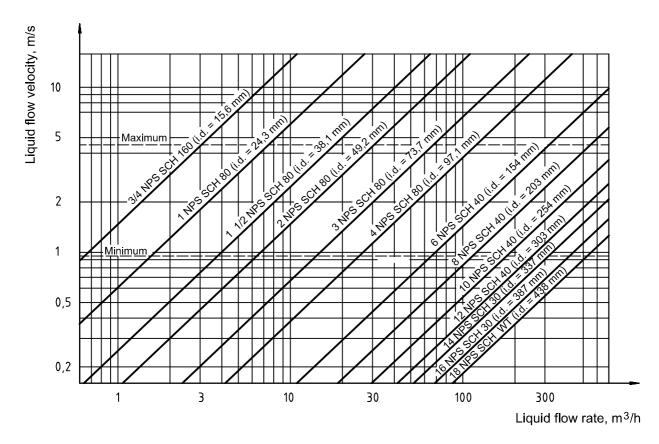
NOTE These curves were determined using equation (2).
