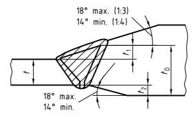
c) Bevel for combined thickness
