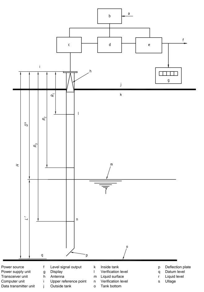
Figure 1 — Example of installation with a still pipe including optional devices
