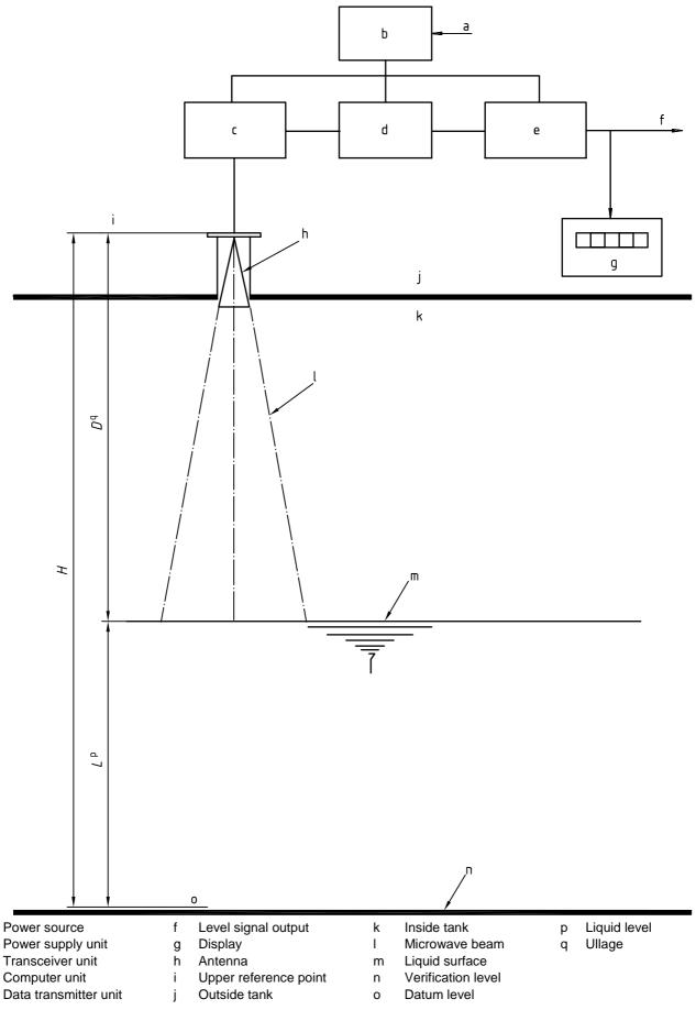
Figure 2 — Example of installation without a still pipe including optional devices
