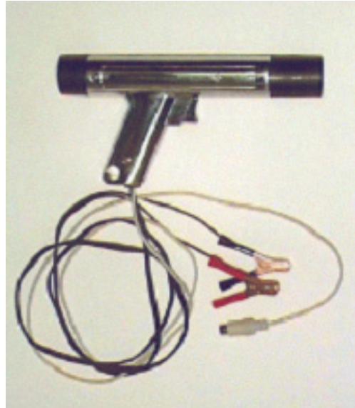
Figure A.3 — Typical stroboscope unit
