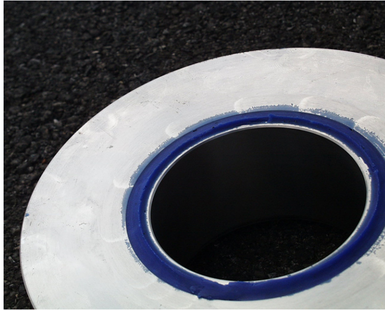
Figure C.2 — Picture of the underside of the in-situ test fixture with a bead of sealing material applied
