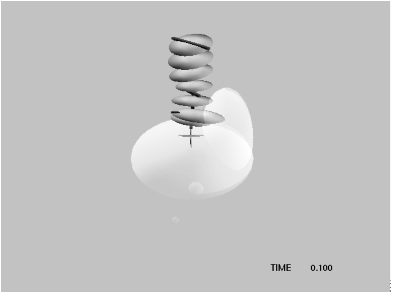
Figure N.7 — Computer simulation of neck torsion test at 0,1 s
