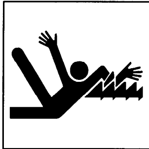
A.8.4 Hand and arm entanglement — Chain or toothed belt drive
