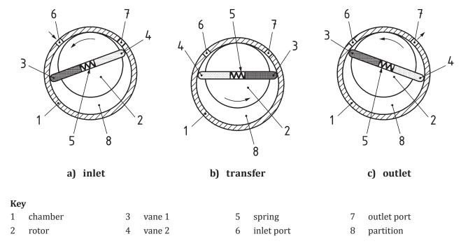
Figure A.2 — Rotary vane pump
