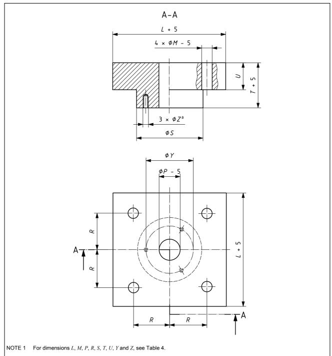
NOTE 2 The tapped holes "Z" are optional and are used for securing the test piece blank to a sub-plate on turning centres having no suitable workholding chuck (i.e. vertical turning centres). In such cases, for proper mounting, the bottom surface of the test piece shall be flat.
