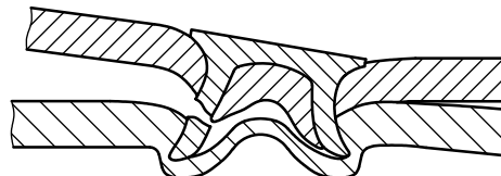
c) Failure of the specimen material
