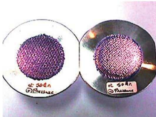
Figure A.2 — Comparative faces of tested test specimens “with pressure” (left) and “without pressure” (right)
