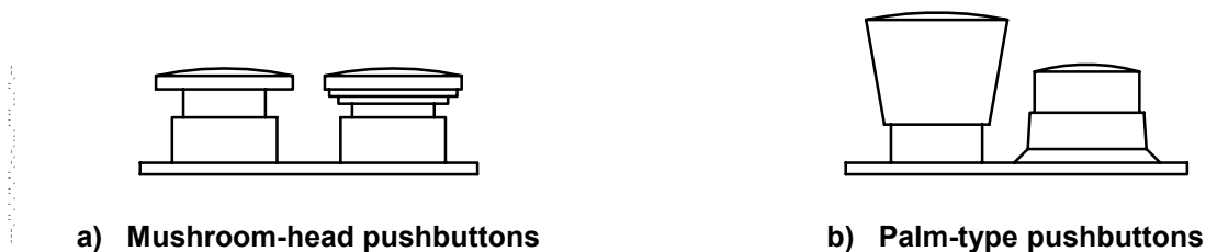
Figure 27 — Types of emergency stop pushbutton
