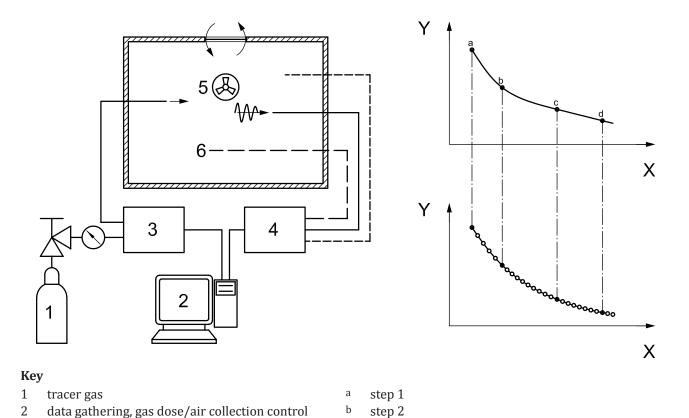
mixing fan X elapsed time concentration measuring by sampling pouch, etc.
