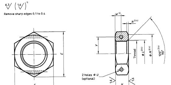
NOTE — Tolerances of form and position shall conform to those specified in ISO 8788.
