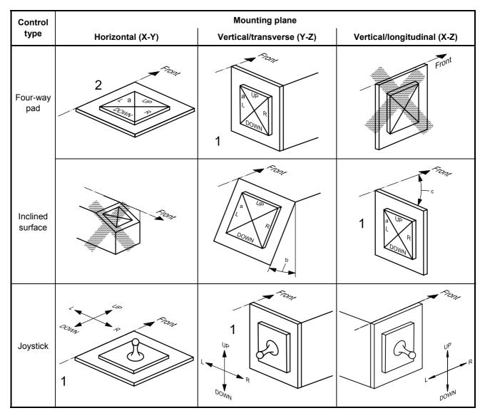
NOTE Unbroken arrows indicate the direction-of-motion for the corresponding field of view motion; the dotted reference line is parallel to the x-axis (front-rear); crossed-out configurations are not recommended.
