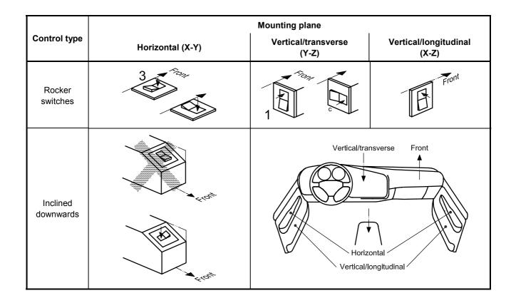
NOTE 1 Unbroken arrows indicate the direction-of-motion for on/increase control; the dotted reference line is parallel to the x-axis (front-rear); crossed-out configurations are not recommended.
