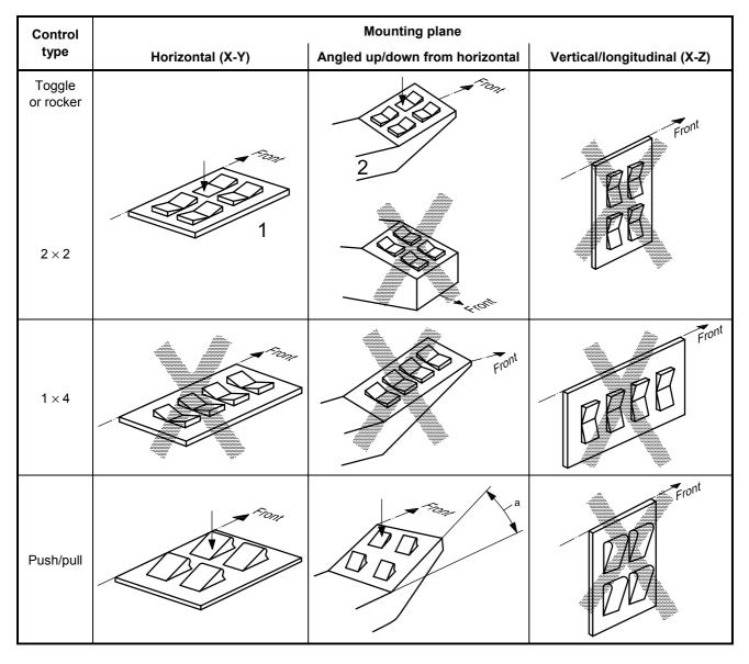
NOTE Unbroken arrows indicate the direction-of-motion to lower the left front window; the dotted reference line pointing to the front is parallel to the x-axis (front-rear) of the vehicle; crossed-out configurations are not recommended.
