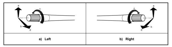
NOTE Unbroken arrows indicate the direction-of-motion for on/increase (turn signal not included).
