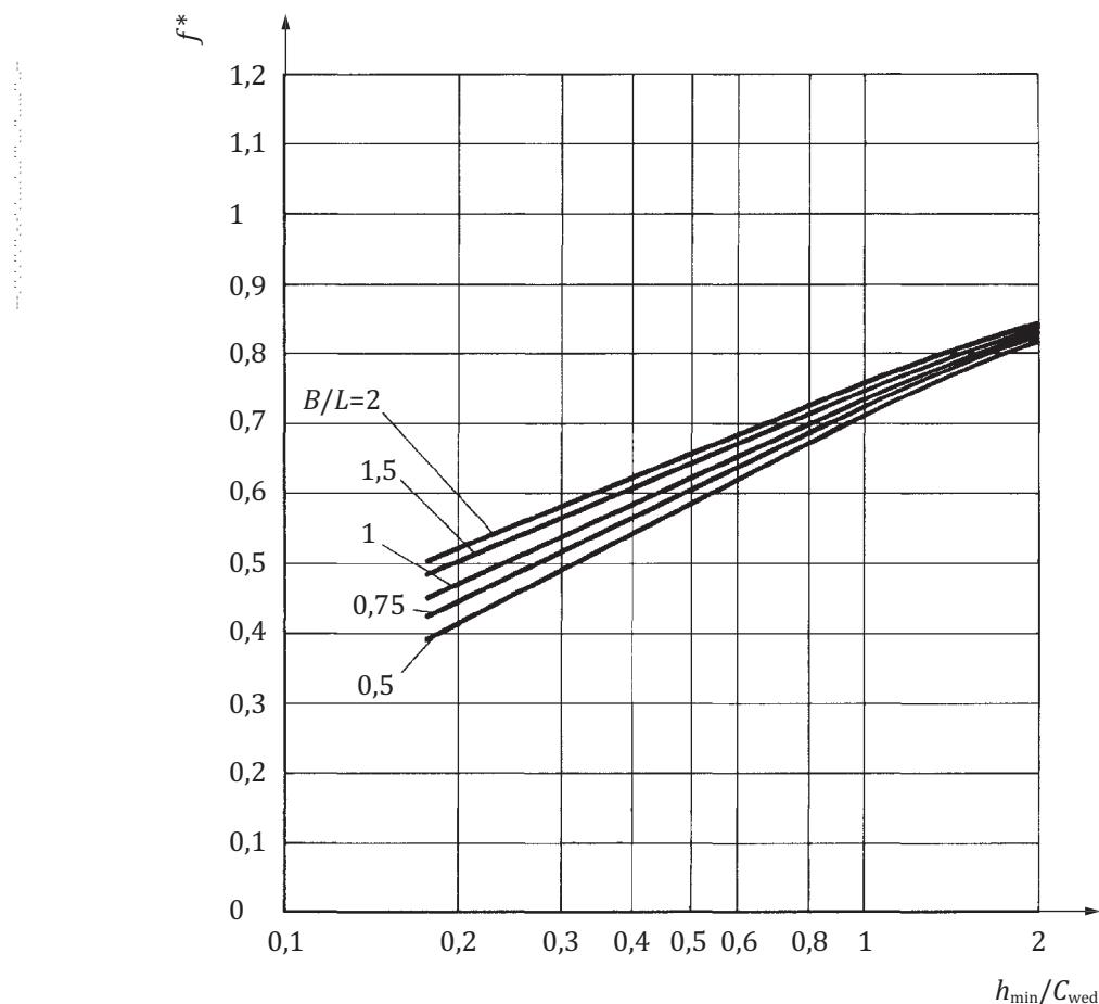
**Figure 2 — Characteristic value of friction,  $f^*$ , as a function of the relative bearing width,  $B/L$ , and the relative minimum lubricant film thickness,  $h_{\min}/C_{\text{wed}}$**
