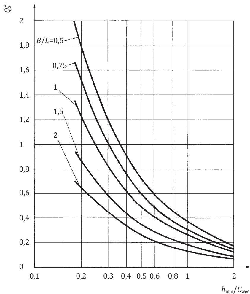
**Figure 4 — Relative lubricant flow rate  $Q_3^*$  as a function of the relative bearing width,  $B/L$ , and the relative minimum lubricant film thickness,  $h_{\min}/C_{\text{wed}}$**
