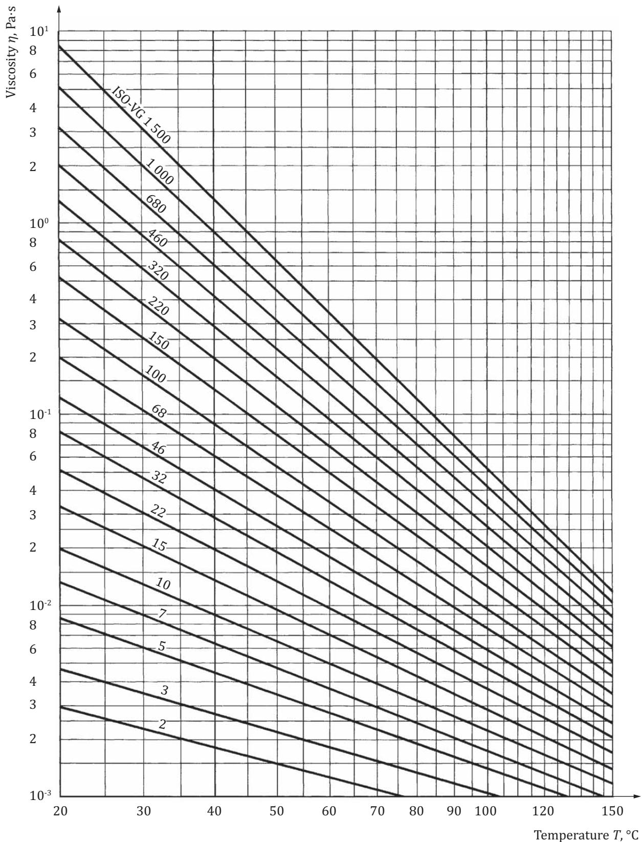
**Figure 6 — Effective dynamic viscosity,  $\eta_{\text{eff}}$ , as a function of the effective lubricant film temperature,  $T_{\text{eff}}$ , at a density  $\rho = 900 \text{ kg/m}^3$**
