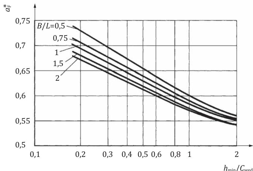
**Figure 5 — Relative coordinate of the pressure centre or supporting point in the direction of motion (circumferential direction),  $a_F^*$ , as a function of the relative bearing width,  $B/L$ , and the relative minimum lubricant film thickness,  $h_{\min}/C_{\text{wed}}$**
