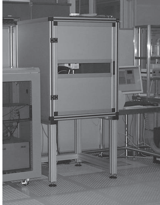
Figure B.1 — AFM in a sound proofing hood consisting of a box of thin aluminium plates, the inside being lined with bitumen and foam combs
