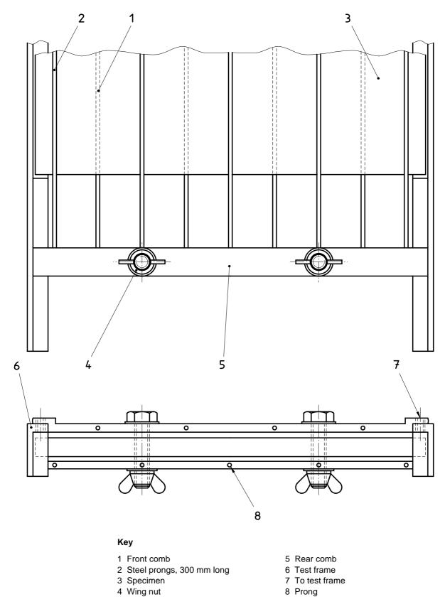
Figure 5 — Typical restraining comb for thermoplastic and flexible materials
