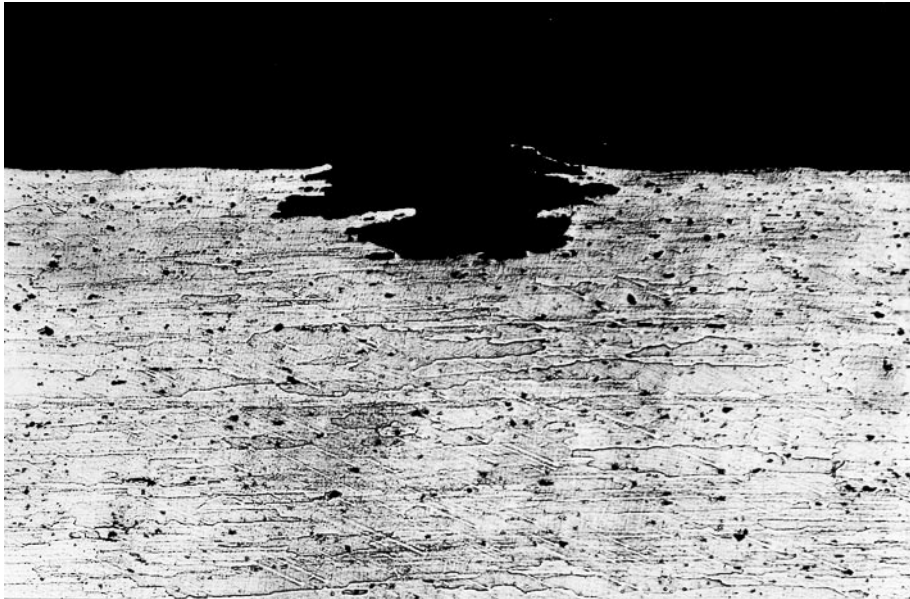
a) Undermining pitting that may from the surface give the appearance of incipient exfoliation.
