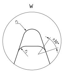
The actual configuration of the tip profile can lie anywhere between the maximum and minimum indicated. Any configuration shall have a transitional radius,  $r_{\rm t}$ , corresponding to a 30° minimum arc tangent to the groove side wall (in accordance with ISO 9981).
