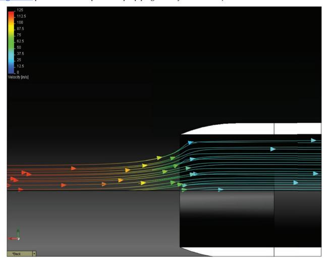
Figure A.1 — Example velocity and flow trajectories
