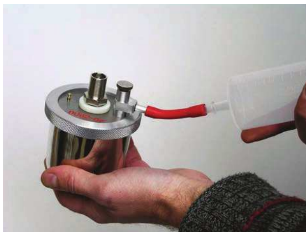
Figure B.1 — Introduction of soil-gas sample into previously evacuated ionization chamber
