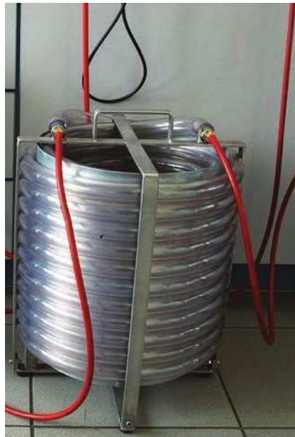
Figure B.3 — Example of radon-220 suppression unit
