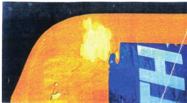
a) Level 1 abrasion damage — Superficial abrasion
