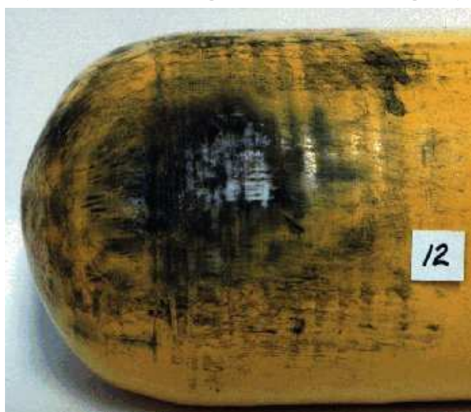
a) Level 1 fire damage — Surface charring only
