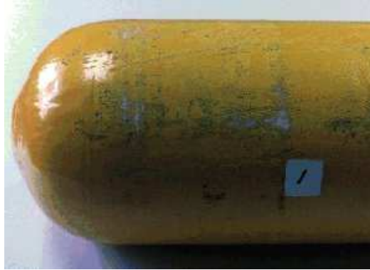
a) Level 1 abrasion damage — Superficial abrasion
