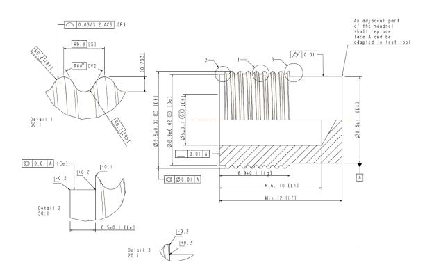
a An adjacent part of the mandrel shall replace face A and be adapted to the test tool.
