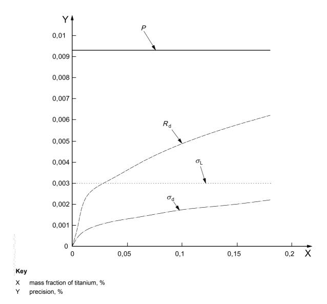
Figure E.7 — Least-squares fit of precision against X for titanium
