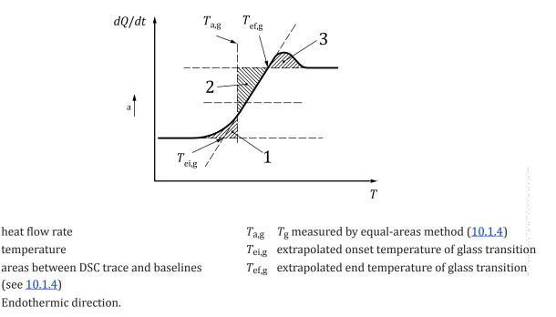
Figure 2 — Example of characteristic glass transition temperature determination according to 10.1.4
