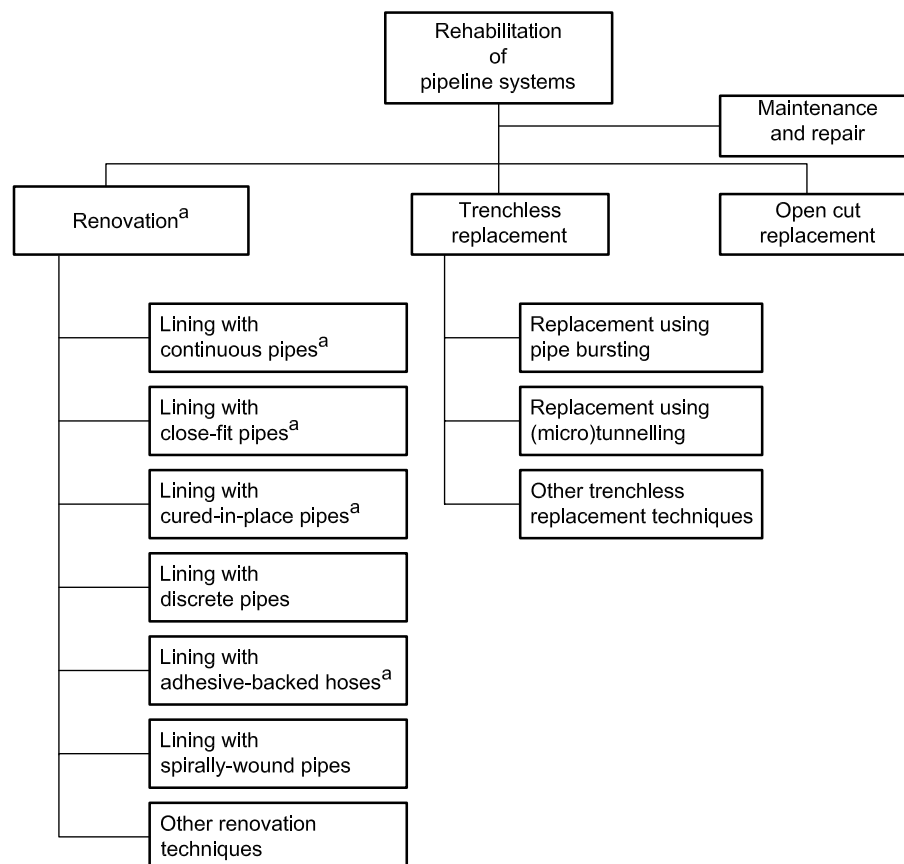
Figure 2 — Technique families for renovation of underground gas supply networks using plastics pipes within the scope of pipeline rehabilitation techniques
