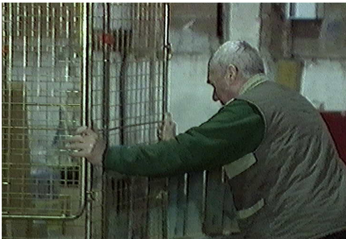
Figure E.1 — Pushing four-wheeled cage over 10 m distance symmetrically with two hands
