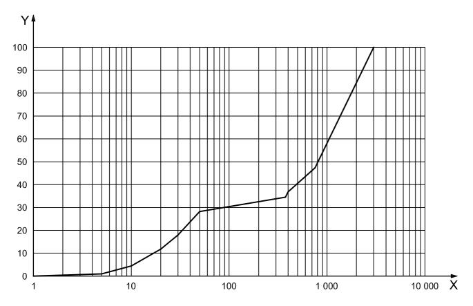
NOTE This particle size distribution was used to determine the mass of particle fractions 1 and 2 of the amalgam sample (see 8.4).
