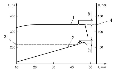
NOTE Figure 2 shows the temperature and pressure versus time graph for a typical autogenous ignition test carried out under nearly constant pressure.
